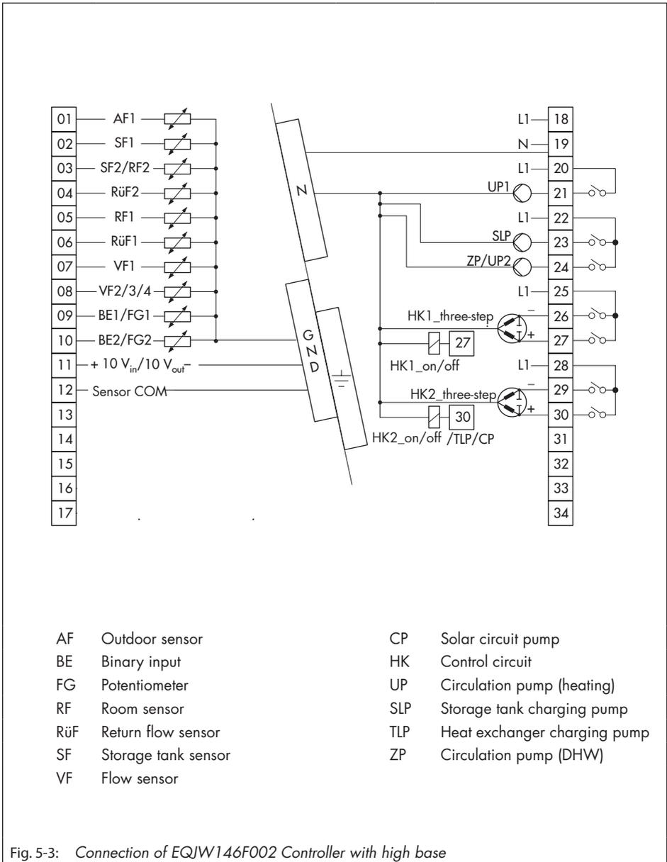
Fig. 5-3: Connection of EQJW146F002 Controller with high base
