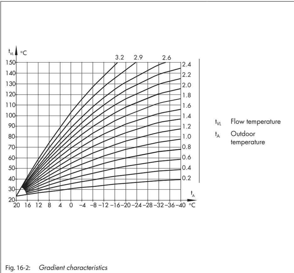
Fig. 16-2: Gradient characteristics
