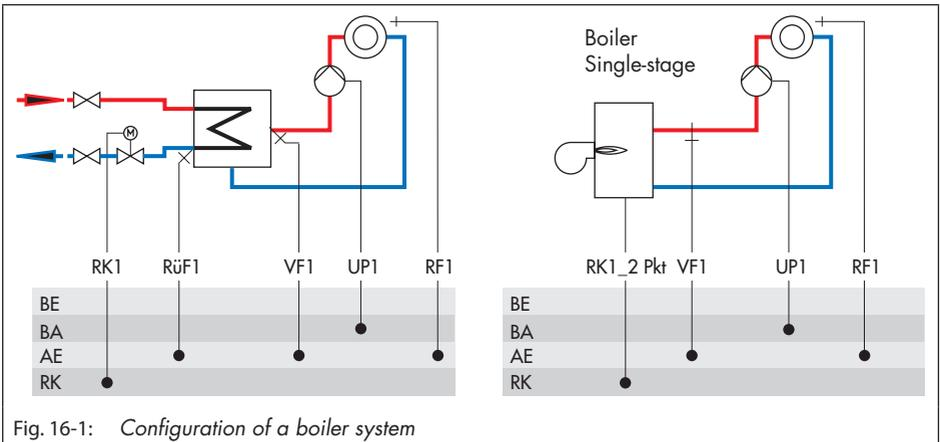
Fig. 16-1: Configuration of a boiler system
