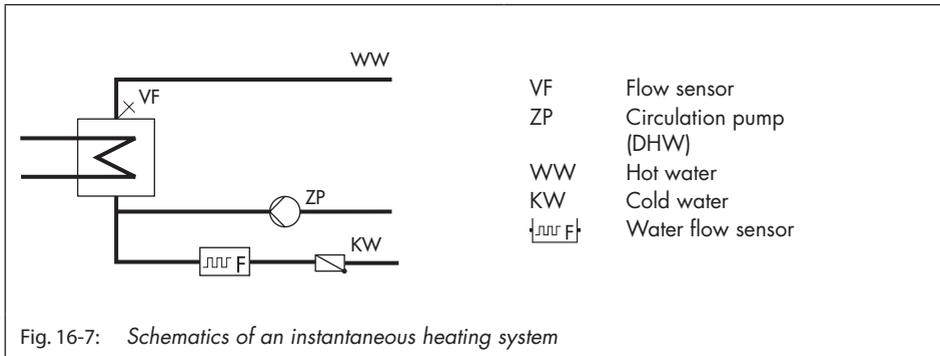
Without flow rate sensor or flow switch, the control of the required DHW temperature at the flow sensor VF is only active during times-of-use of the circulation pump ZP. The water flow sensor or flow switch allows the controller to recognize when DHW tapping starts and stops. Control of the required DHW temperature can be made to be active only during DHW tapping by deleting all times-of-use of the circulation pump.
