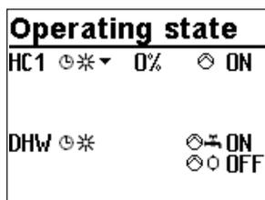
Turn the rotary switch to ☾✱ (operating modes). The operating states of all system control circuits are displayed:
