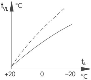
The gradient needs to be increased if the room temperature drops when it is cold outside.
