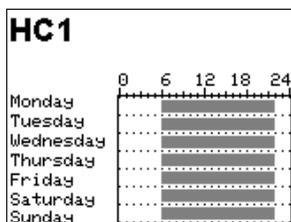
Turn the rotary switch to
