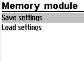
The memory module is plugged into the RJ-45 connector socket located at the side of the controller. Once the module has been connected, 'Save settings' appears on the controller display. If the memory module already contains data from a different EQJW146F002 Controller, turn the rotary pushbutton until 'Load settings' is displayed.
