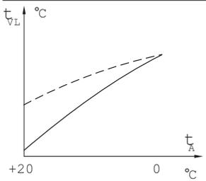
The level needs to be increased and the gradient decreased if the room temperature drops when it is mild outside.
